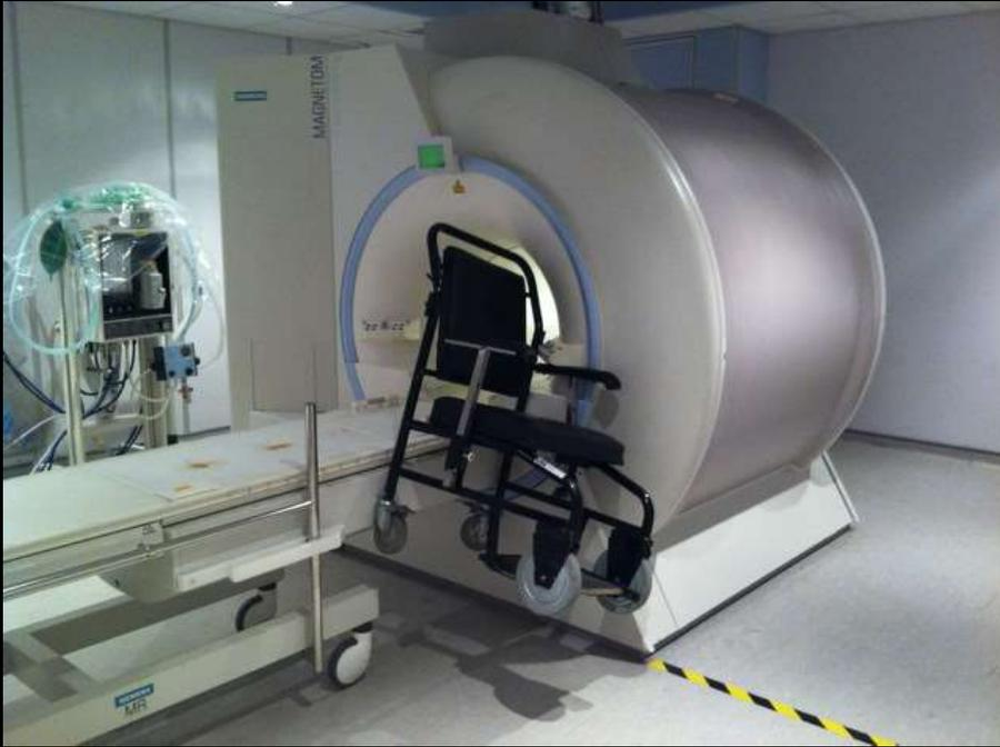
Fortunately, nobody was injured in this case but this wheelchair will have been attracted to the magnet at around 30 miles per hour. The field is generally never switched off in a superconducting magnet, which is why it cost £20,000 pounds to switch off the magnet, remove the wheelchair and power it up again, as well as repairing the damage to the covers surrounding the magnet.
