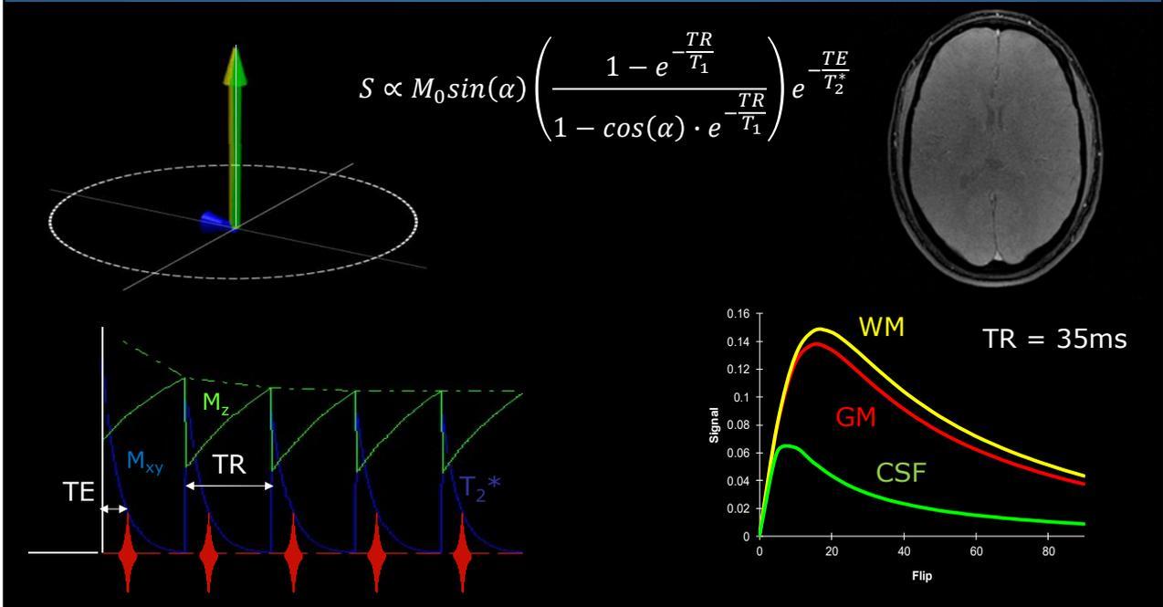
Here we can see the effect of a reduced flip angle excitation. Note that the signal behaviour is now a function of TE, TR and flip angle as shown in the slightly more complicated signal equation. The images show the effect of increasing the flip angle from 10°-90°. Note the changing contrast and decreasing SNR as the flip angle is increased.
