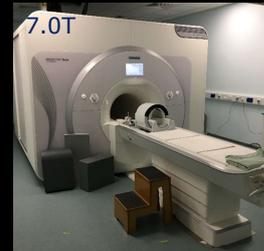
The 0.4T magnet uses permanent magnet pole pieces. The 0.6T electromagnet is an iron-cored electromagnet that weights over 100T. The 0.5T  $MgB_2$  magnet is cryogen free using two Gifford-McMahon cryocoolers operating at 20K to mechanically keep the system operational. The 7.0T system uses Niobium Titanium windings at 4.2K
