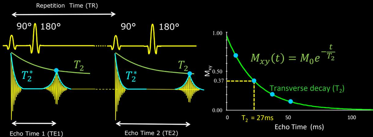
It would be possible to calculate the  $T_2$  relaxation constant by acquiring signals with different TEs. However the TR needs to be kept as long as possible to minimise the  $T_1$  effect on the measured signals. The blue circles show the echo amplitudes at different TEs from which the  $T_2$  decay constant can be calculated.
