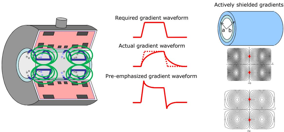
The rapid switching of the gradients induces eddy currents in nearby conducting components of the magnet cryostat. These persist for varying durations depending on the resistivity of the metal involved. The field generated by the eddy currents combines with the intended gradient field to create waveform distortions, which can result in image artifacts and signal loss.
