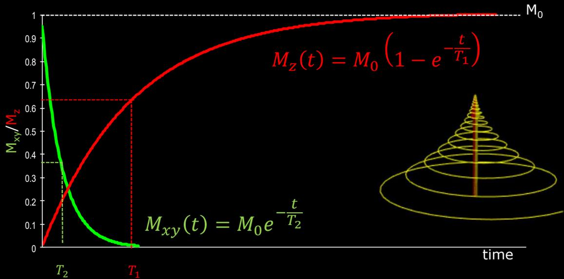
This figure shows the longitudinal magnetization recovery (red) and transverse magnetization decay (green). The  $T_1$  is the time for 63% of the magnetisation to have recovered, whilst the  $T_2$  is the time for 37% of the magnetisation to have decayed.
