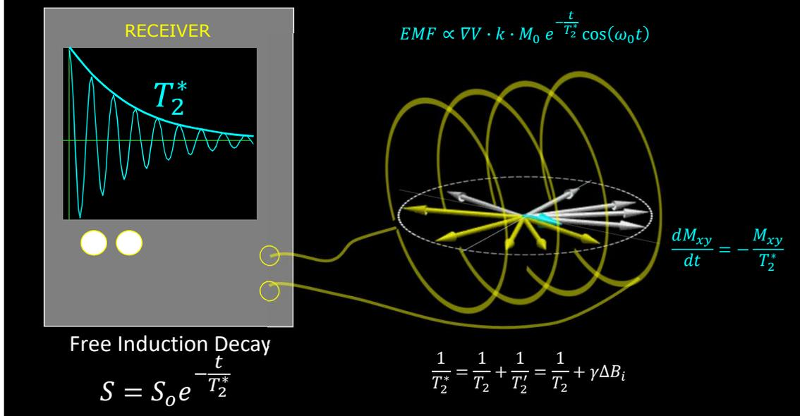
Static version of the previous slide showing near complete transverse dephasing.
