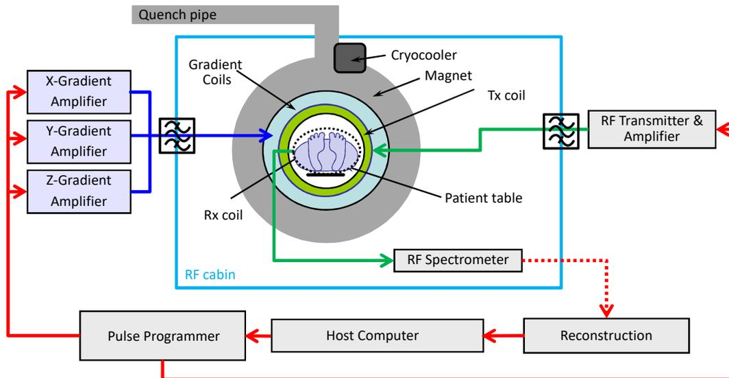
The diagram provides an overview of an entire MR system. The red lines represent digital signals, whilst the green lines represent the analogue RF transmit/receive signals and the blue lines the analogue gradient waveforms. The dotted red line is fibre-optic.
