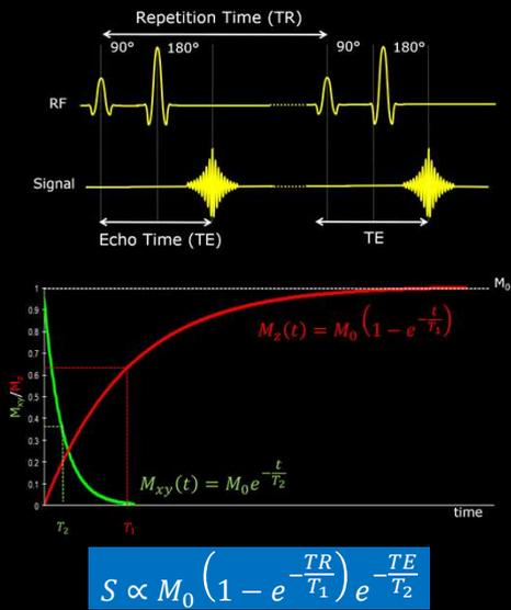
$$S \propto M_0 \left(1 - e^{-\frac{TR}{T_1}}\right) e^{-\frac{TE}{T_2}}$$
