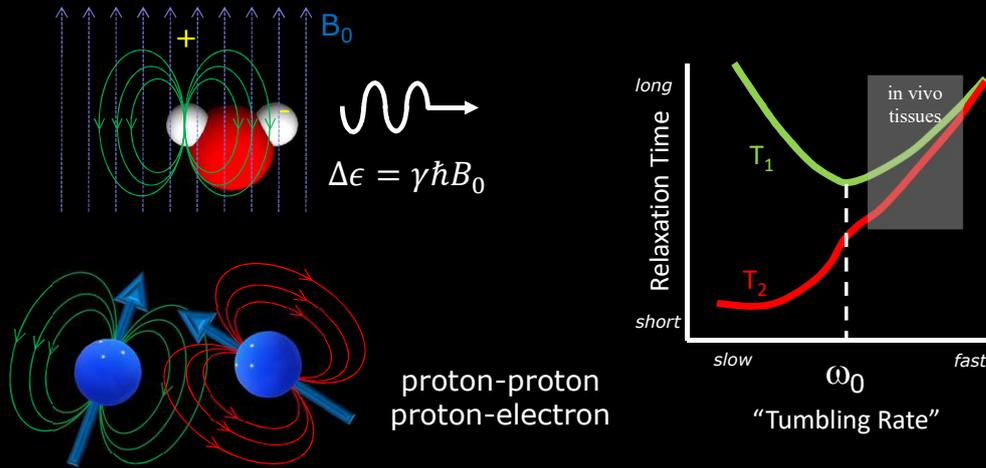
The alternating field comes from neighbouring protons or other nuclei or molecules, which have magnetic moments. In water the nearest adjacent nucleus will be the other hydrogen atom on the same molecule. Therefore, relaxation will primarily arise through the magnetic moment that one hydrogen nucleus 'sees' as it tumbles relative to the moment of the other hydrogen nucleus. This is often called an intra-molecular dipole-dipole interaction.
