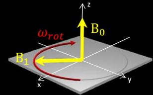
$$\frac{dM_x}{dt} = \gamma(M_y B_0 + M_z B_1 \sin(\omega_{rot}t))$$
