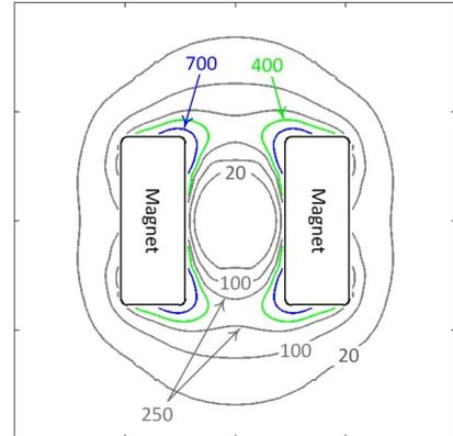
In this example, there is no path into the magnet that does not pass through the "entry SG" contour of 250 G/cm (2.5 T/m)
