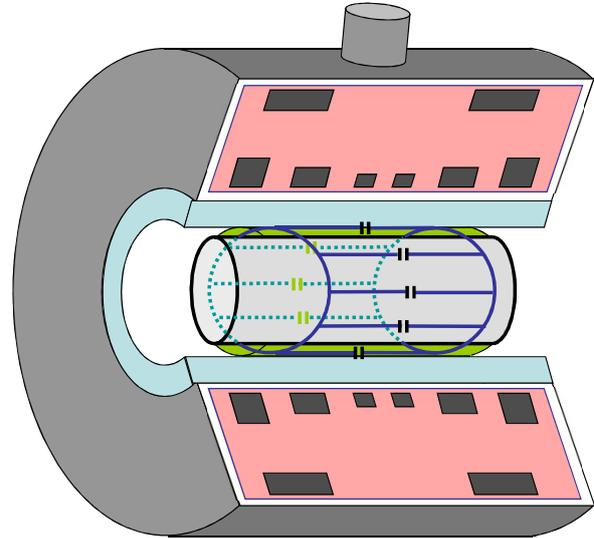
The purpose of the RF transmit coil is to create the circularly polarised time-varying  $B_1$  field at right angles to  $B_0$ . A large diameter birdcage “body” coil is generally used since this creates the most spatially uniform  $B_1$  field. The coil is a resonant circuit tuned to the Larmor frequency for the given field strength and impedance matched to the RF power amplifier.
