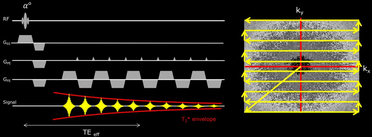
Although this is a gradient echo EPI sequence, i.e. the readout is immediately following an  $\alpha^\circ$  RF pulse and not a  $90^\circ$ - $180^\circ$  spin echo EPI – the echo-planar readout trajectory is the same in both cases. The animation demonstrates the raster style k-space trajectory. The phase encoding gradient is blipped to move up one k-space line whilst the frequency encoding gradient alternates in polarity so the echoes are alternately readout forward and backward.
