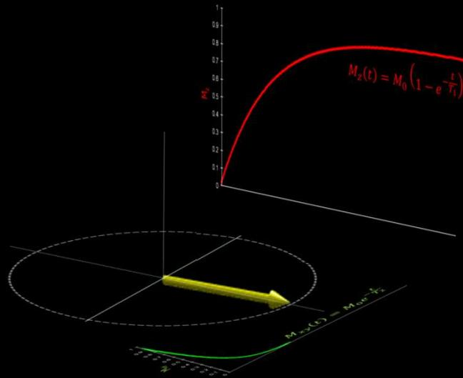
This figure shows the longitudinal magnetization recovery (red) and transverse magnetization decay (green) in the laboratory frame. In biological tissue  $T_2$  is approximately an order of magnitude shorter than  $T_1$ , i.e. For brain white matter the  $T_1$  is around 560ms and  $T_2$  is around 90ms. Remember that  $M_0$  is proportional to the proton density  $\rho$ .
