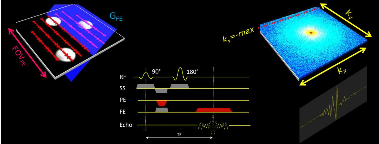
The y-direction phase shift induced by the PE gradient is retained during the formation of the echo in the presence of the FE gradient. In our 2D k-space this “line” of echo data will be assigned to the top of the raw data matrix, since it is acquired with maximum phase encoding, i.e.  $k_y = -\text{max}$ .
