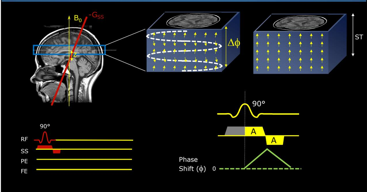
The phase shift across the slice can be reversed by the application of an opposite polarity pulse with an area equal to the area of the gradient from under the magnetic centre of the RF pulse to the end of the gradient. Without this rephasing gradient the signal across the slice would be totally dephased and you wouldn't see anything.
