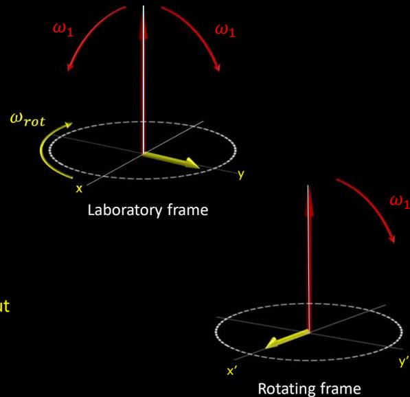
Comparison of laboratory (fixed) and frame rotating at  $\omega_{rot}$  behaviour. It is much easier to work in the rotating frame.
