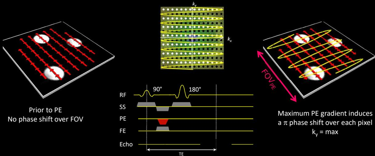
We can see that this maximum negative PE gradient has caused a  $\pi$  phase shift to be induced over each pixel. This represents the highest possible spatial frequency and hence the spatial resolution of the image in the y-direction.
