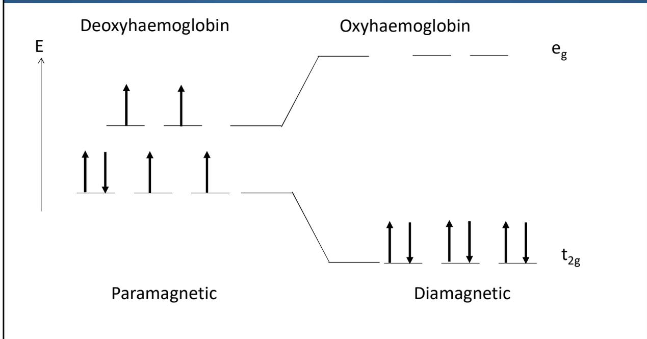
Deoxyhaemoglobin (Hb) is paramagnetic whereas oxyhaemoglobin (HbO<sub>2</sub>) is diamagnetic. Paramagnetism causes a shortening of the T<sub>2</sub><sup>\*</sup> relaxation time in comparison to diamagnetism. Activation of a brain area, e.g. the motor cortex results in an increase in HbO<sub>2</sub> above the metabolic need. There is therefore a surfeit of HbO<sub>2</sub> and hence an increase in signal intensity on T<sub>2</sub><sup>\*</sup>-weighted gradient echo.
