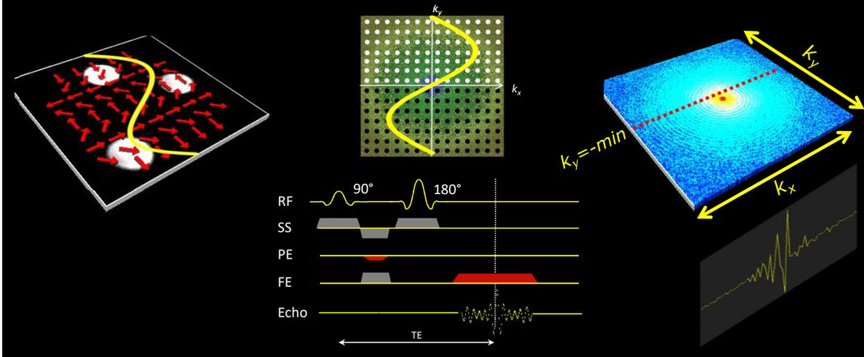
We can see that this minimum negative PE gradient has caused a  $2\pi$  phase shift to be induced over each pixel. Following frequency encoding in our 2D k-space this "line" of echo data will be assigned nearest the centre of the raw data matrix, since it is acquired with minimum phase encoding, i.e.  $k_y = -\min$ .
