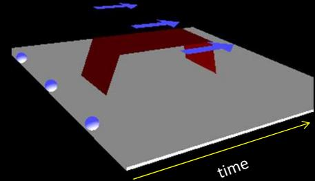
$$\Delta\phi = \gamma \int_{t=0}^{t=T} G_x x dt$$
