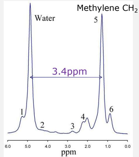
Essentially the protons in fat precess 3.4ppm slower than water due to magnetic shielding of the orbital electrons. So at 1.5T this results in a frequency difference of  $64\text{MHz} * 3.4\text{ppm} = 220\text{Hz}$
