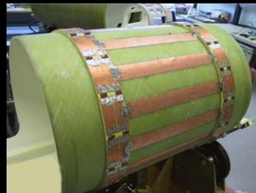
RF transmission involves mixing the digitally generated RF pulse envelope (which dictates the bandwidth of the excitation pulse) with the slice select frequency. This analogue waveform is amplified and applied in quadrature to the birdcage body coil in order to generate a circularly polarised RF that rotates in the same sense as the precessing nuclear magnetisation.
