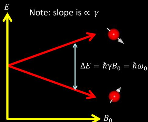
From a QM perspective the energy difference between the two orientations in a static magnetic field of  $B_0$  is given by  $\Delta E = \gamma\hbar B_0$ , and is exactly equivalent to the classical Larmor equation.
