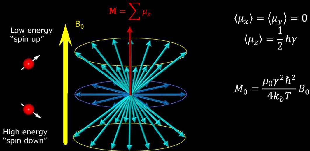
Water contains  $6.67 \times 10^{22}$  protons  $\text{ml}^{-1}$ . So at body temperature at 3.0T we get  $M_0 \approx 0.02 \mu\text{Tml}^{-1}$ . Assuming the human head has volume of 1500ml and is approximately 80% water we get  $M_0 \approx 20 \mu\text{T}$
