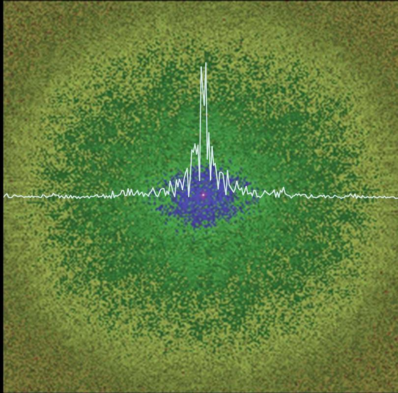
The real signal from a human subject looks like this and can be displayed as one line of a raw data image it looks like this. Now the complete MRI scan involves changing these gradients many hundreds of times and detecting the signals across the entire body. So the scanner acquires data like this. This is the raw data, sometimes called  $k$ -space.
