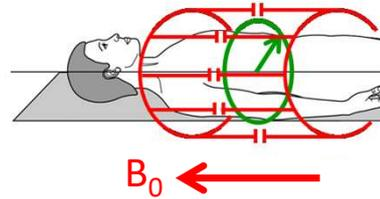
Vertical or horizontal field systems can use simple solenoids to create  $B_1$  since  $B_0$  is orthogonal. In superconducting magnets where the field is horizontal the coils need to be of the birdcage design.
