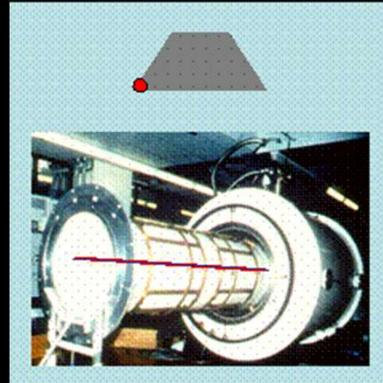
The physical  $G_x$ ,  $G_y$  and  $G_z$  gradients are mapped to the logical slice select, phase encoding and frequency encoding gradients. This enables images to be obtained in any orthogonal plane or a combination of two or three allow imaging in a single or double oblique plane. The gradients physically flex when they are pulsed, like a loudspeaker, resulting in the characteristic knocking noise associated with MRI.
