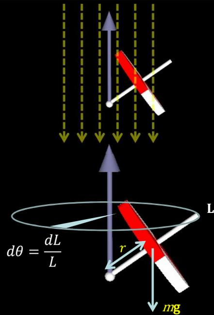
A gyroscope, under the influence of gravity, will precess about the vertical.
