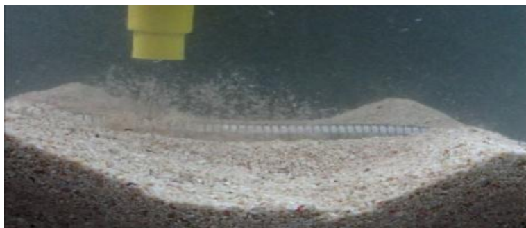
(e) A few passes are made over the central section of the pipeline between the 2 crests.
