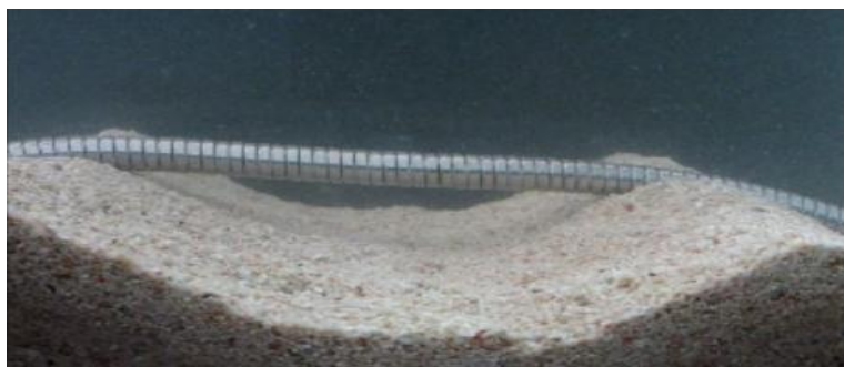
(a) Free span section of pipeline.
