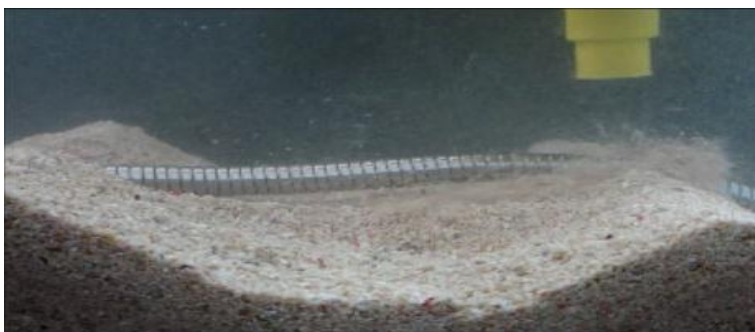
(c) The Mass Flow Excavator (MFE) is used to fluidize the sand at the right crest. This causes the pipe on the right crest to settle lower into the sand.
