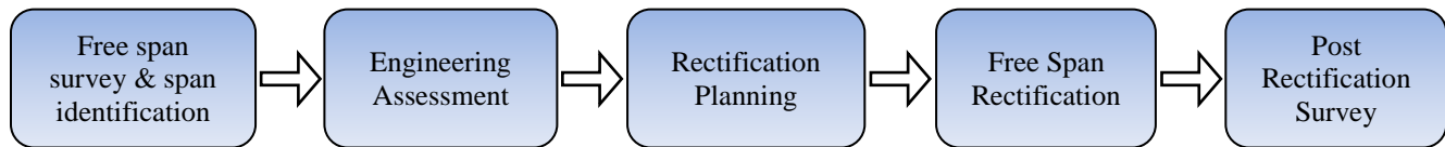
Figure 3: Typical Free span rectification process
