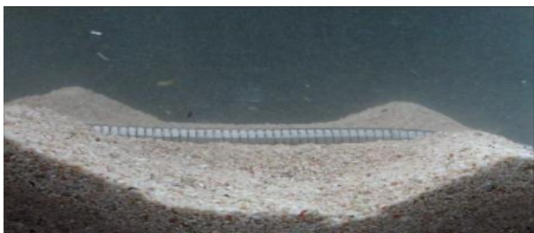
(f) Pipeline is fully supported by the sand and there is no more free span.
