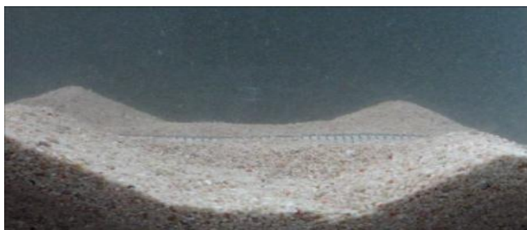
Figure 6 (a to h): Demonstration of Pipeline Lowering (PL) in a small scale setup.
