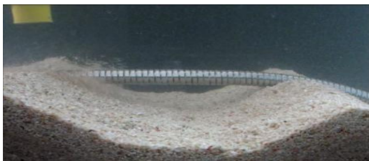
(b) Small scale model of Mass Flow Excavator (MFE) is used to fluidize the sand at the left crest. This causes the pipe on the left crest to settle lower into the sand.
