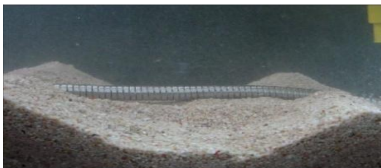
(d) Pipeline has been lowered at both the crests.
