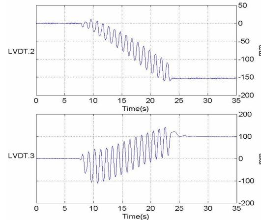
Fig. 6b. Clay liner & soil surface motion during EQ.2
