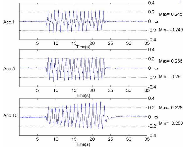
Fig. 4b. Accelerations during EQ.2
