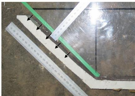
Fig. 9. Post-test cross section of the clay liner.
