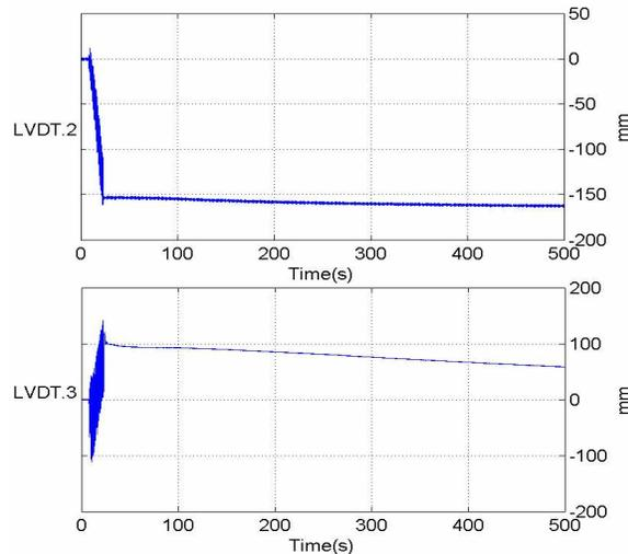
Fig. 7b. Clay liner & soil surface motion after EQ.2
