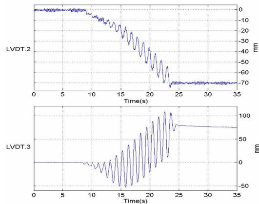
Fig. 6a. Clay liner & soil surface motion during EQ.1
