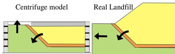
Fig. 7c. Clay liner motion in model vs in real landfills
