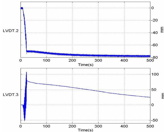
Fig. 7a. Clay liner & soil surface motion after EQ.1
