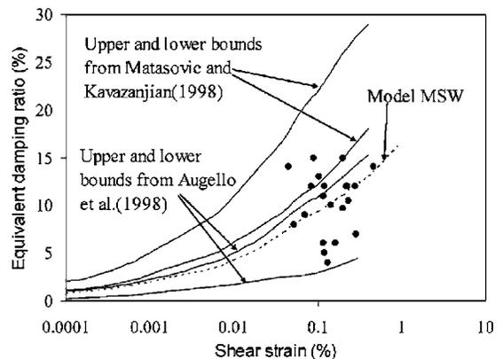
FIG. 12—Equivalent damping ratios of model waste.
