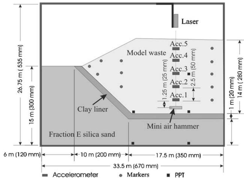
FIG. 1—Cross section of IT-01 model (model scale dimensions in brackets).
