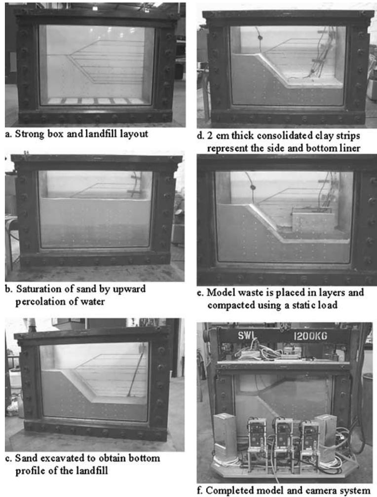
FIG. 2—The sequence of model preparation.
