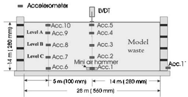
FIG. 6—Cross section of IT-02 model (model scale dimensions in brackets).
