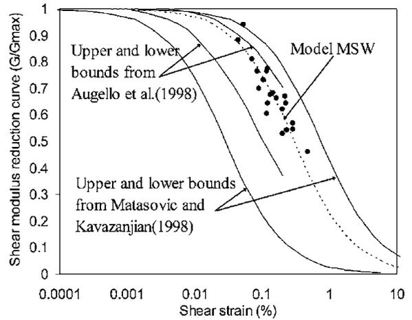
FIG. 11—Shear modulus reduction curve of model waste.
