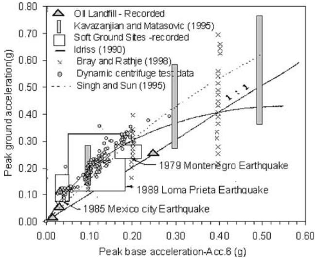
FIG. 9—Comparison between recorded, numerical, and dynamic centrifuge data.
