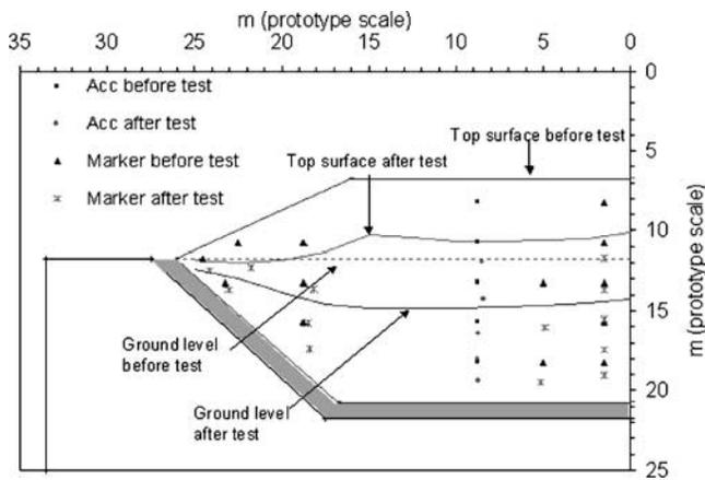
FIG. 4—Settlement profile of the landfill model from IT-01 test.
