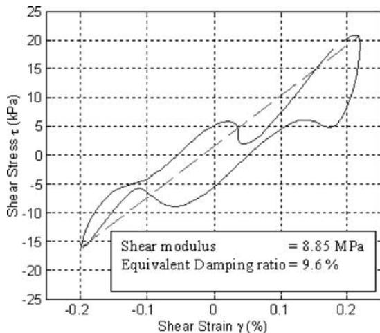
FIG. 10—Stress-strain loop of model waste obtained from Acc. 6, 7, and 8 of E.7
