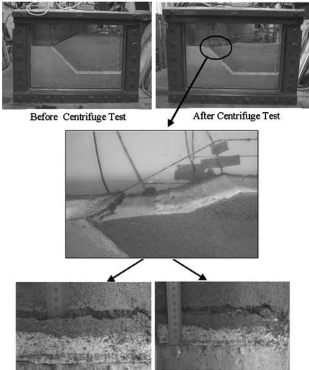
FIG. 5—Posttest observations of settlement induced cracking in waste side liner.
