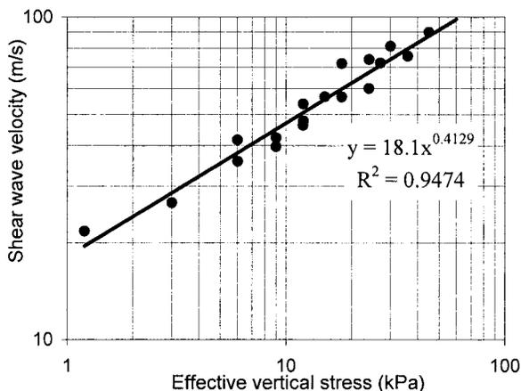
FIG. 3—Relationship between shear wave velocity and vertical effective stress.
