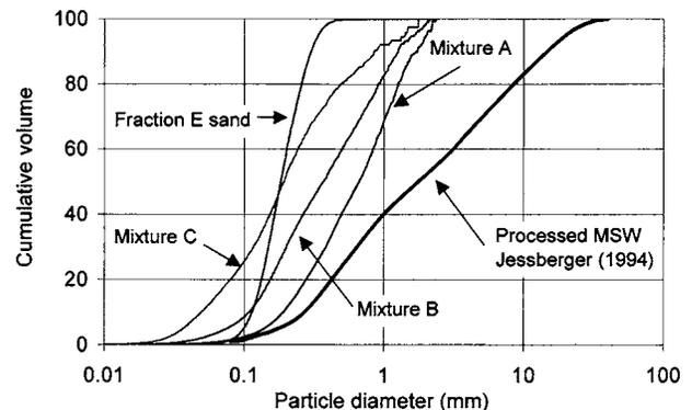
FIG. 5—Particle size distribution of model waste mixtures.
