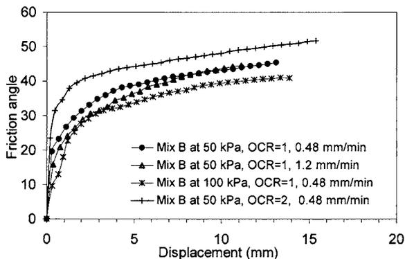
FIG. 6—Strain rate and overconsolidation ratio (OCR) effects on shear strength of Mixture B.
