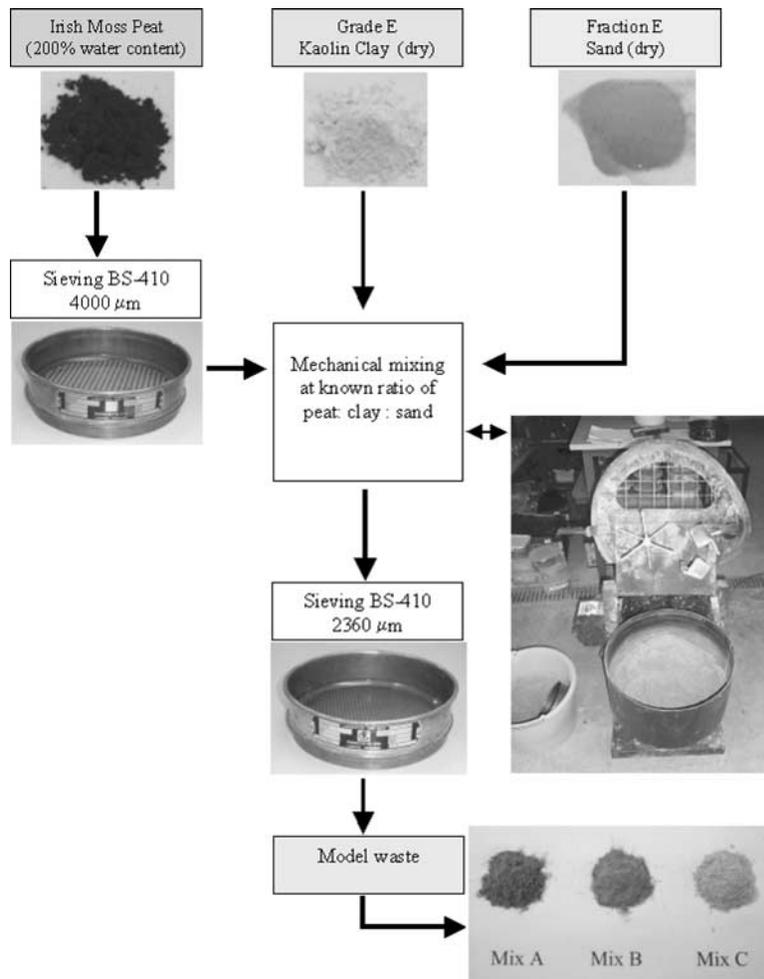
FIG. 1—Preparation of model waste mixtures.
