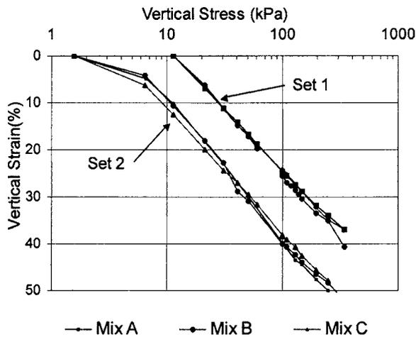
FIG. 3—Vertical strain vs vertical stress for model waste mixtures.
