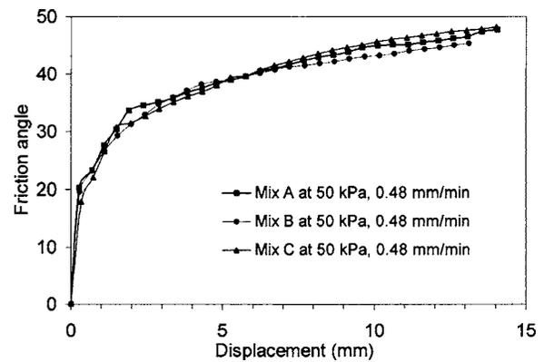
FIG. 4—Shear strength of model waste mixtures.
