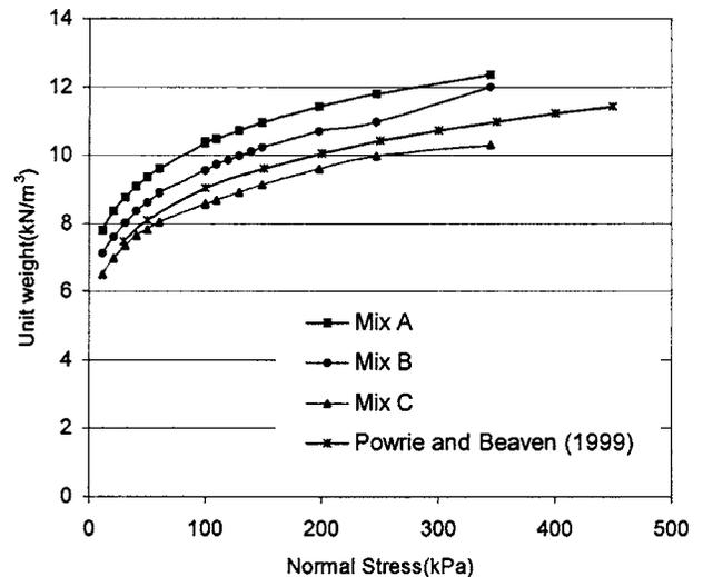
FIG. 2—Variation of unit weight with vertical stress for model waste mixtures.
